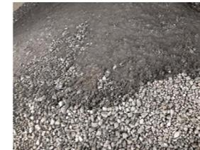
Prior to the improvement: Large amount of fine coal particles causes boiler slagging
